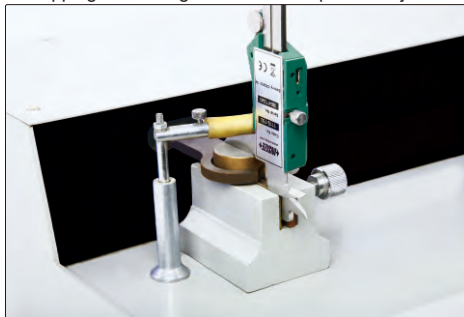
lapping measuring surfaces of caliper lower jaws
